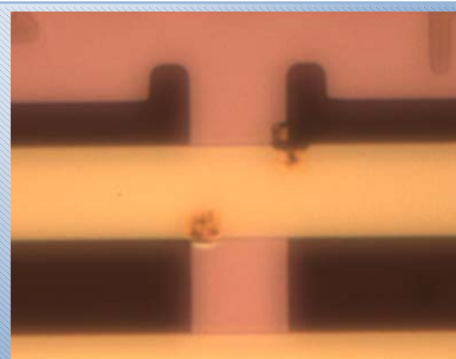
Welding Power line (688). 50X
